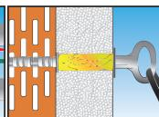
Set the washer aligned to the wall. Installation completed
