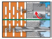
Drill the insulation panels with a cup Clean the hole by using proper with a centering tip. Drill the masonry cleaning brushes and pump with a Ø18 drill bit
