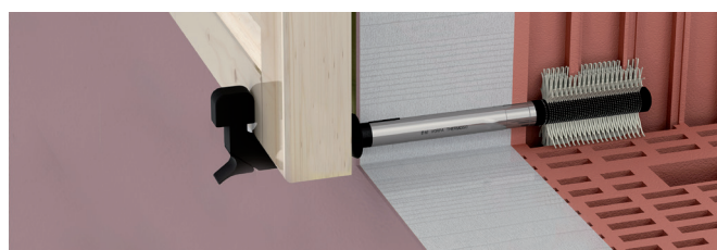
CVX N black plastic perforated sleeve to be used with THERMOISO PLUS on hollow materials for insulated walls
