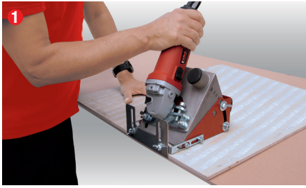
1 Engraving slab by grooving tool Click-Cut
