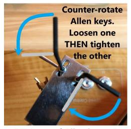
1/4 turns of Allen key = 1 degree azimuth shift
