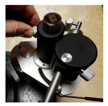
Just a quarter of a revolution of the lock screw -  $90^{\circ}$  - is enough.
