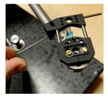
The AQUILAR's mirrored alignment template ensures a super precise 1-point alignment to the UNI-DIN tangential curve.
