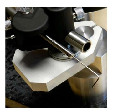
Now please take the HD18 counterweight and slide it - narrow head to the front - onto the stainless steel counterbar till it reaches the ball head in the top of the counterbar.
