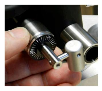
Next rotate the counterweight clockwise till the desired tracking force in grams shows at the 12 o'clock position.
