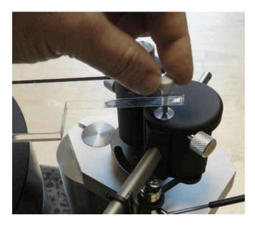
Now slide the alignment template into place with the M4 thread at the end of its outward positioning beam over the pivot locating plate on the AQUILAR.
