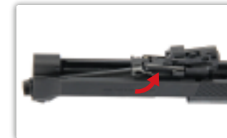
Remove the recoil spring and guiding rod.
