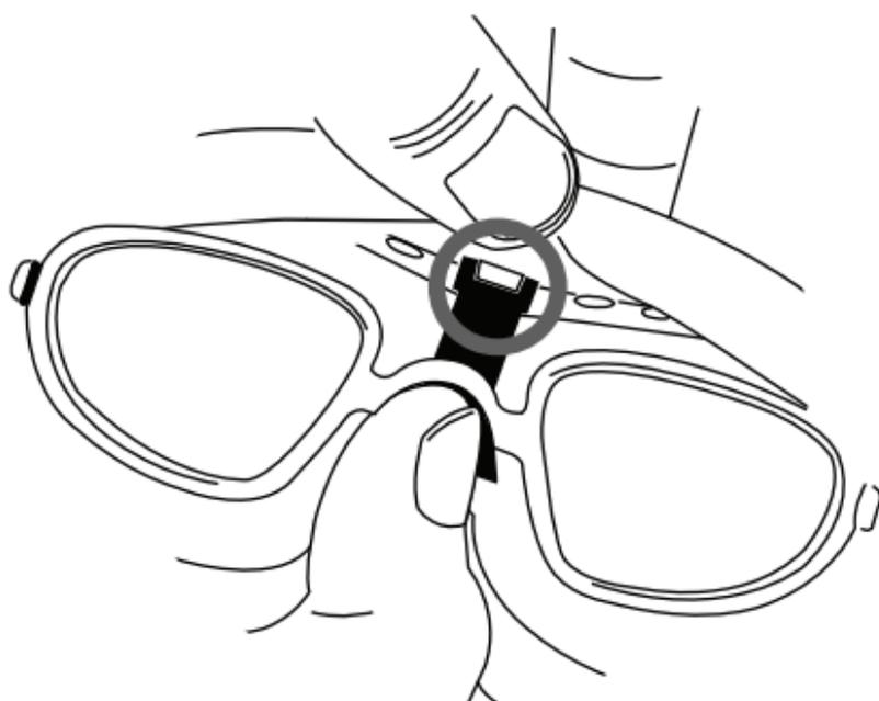
Lift the frame to allow easy access to insert the adapter into the frame.
