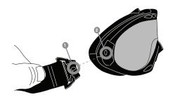
The goggle strap is secured to the goggle by inserting the goggle strap pin at (1) into the goggle face frame at (2).
