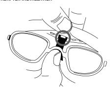
Lift the frame to allow easy access to insert the adapter into the frame.
