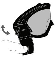
Remove or attach goggle strap by positioning the strap perpendicular to the frame as pictured above.
